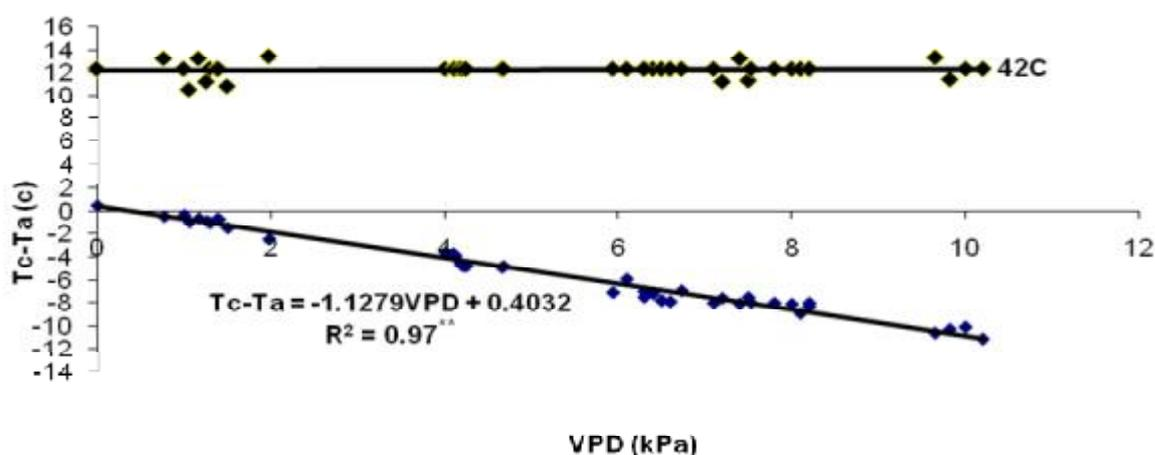
Figure 1. Stressed and non-stressed baselines for calculation of CWSI in turfgrass
